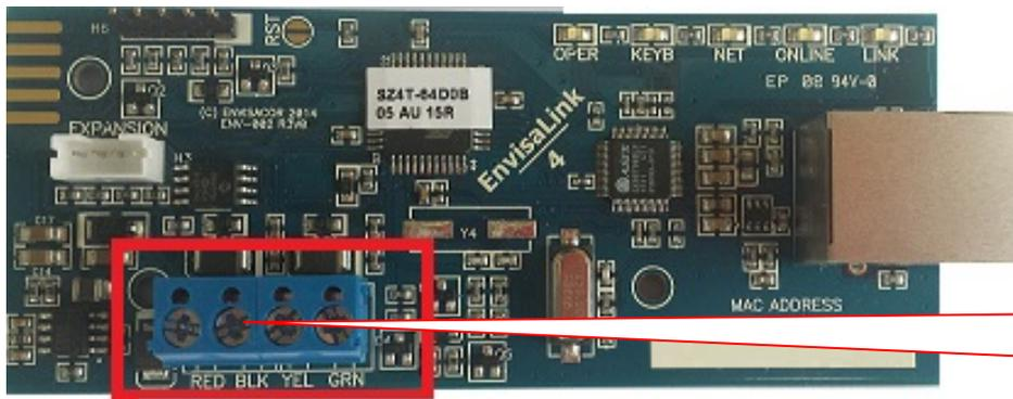
Connect the power supply leads to the terminals on the **Envisalink4**: Red and Black terminals.
